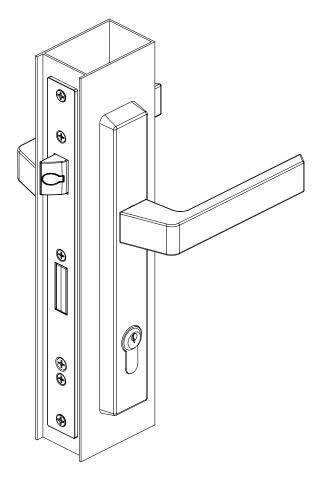
Note: If cylinder turn knob, key or lever is difficult to turn, lift or depress, inspect the alignment of strike plates.
