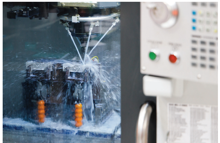
Manufacturing of a mortice lock case using the CNC machine.
