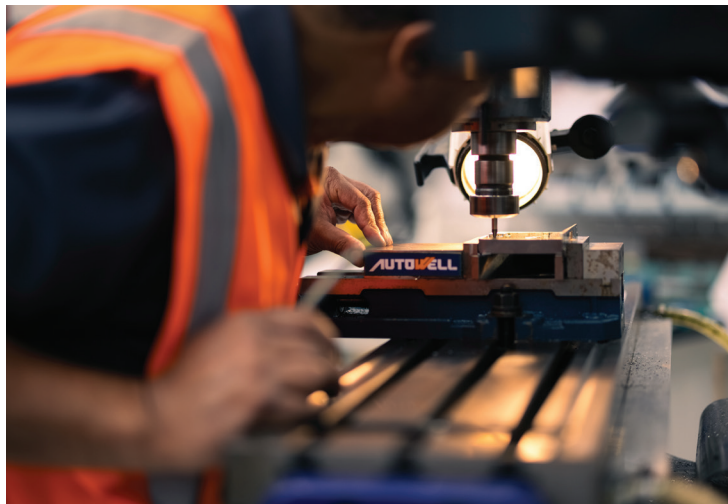
Prototyping using a milling machine for testing of a mortice lock case
