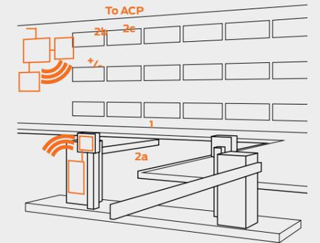
The GCK400 wireless gate kit is ideal for upgrading to real time access control on garage and parking lot entries. The GCK400 kit features open architecture devices and is compatible with popular Wiegand and Clock & Data format readers.
