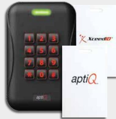
With aptiQ multi-technology readers your customers can use either proximity, smart cards or an NFC-enabled smart phone in their existing system. This allows for an easy transition to upgraded technology over time and as budgets allow.
