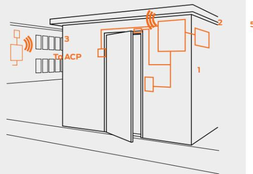
The WRI400 has a communication range of up to 1,000 ft. with clear line of sight. Remote antennas can be used to increase the range when needed. The WRI400 eliminates the need to dig a trench to the storage shed, saving time and money associated with equipment rental and running wires under ground.
