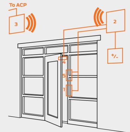
The WRI400 wireless reader interface is a networked access point controller designed to provide wireless connectivity to traditional electronic access control components, including standard Wiegand readers, door position, tamper, and request to exit switches.
