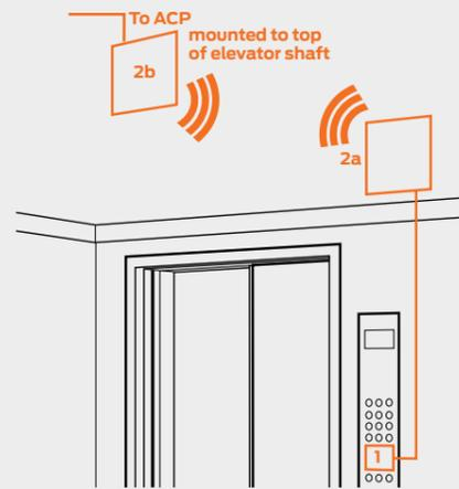
The ECK400 wireless elevator kit is ideal for retrofit applications, it eliminates the need to run traveling cables inside the elevator shaft. The reader is connected to the WRI400 on top of the cab. The WRI400 communicates over 900 MHz to the PIM400 on top of the shaft. The PIM400 is wired back to the ACP for real time monitoring.
