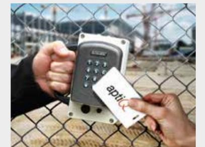
The WPR400 can validate credentials in real time when in range of the PIM400-TD2, which is connected to the access control panel. The WPR400 is capable of operating in cache mode, and when enabled, it keeps a local database of valid access grants. Upon moving the WPR400 to a location that is out of range the local database can be used to verify up to the last valid 1,000 users.
