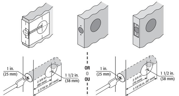
**3.2** Prepare the door jamb - using the strike plate as a pattern, drill the latch and screw holes, and chisel out a mortise until the strike plate fits flush. To assure proper lock function, the holes in the door jamb must be drilled 28mm deep.
