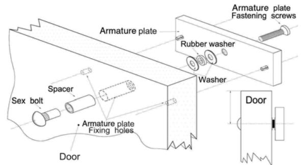
ARMATURE PLATES MUST BE FIXED AS SHOWN ABOVE. DO NOT OVER TIGHTEN THE FIXING SCREW. THE ARMATURE MUST BE ALLOWED TO 'FLOAT' ON THE RUBBER WASHER.
