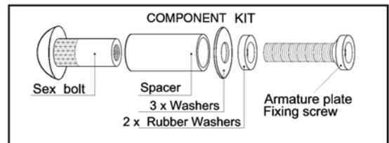
ARMATURE PLATES MUST BE INSTALLED WITH THE COMPONENTS SHOWN ABOVE. THESE COMPONENTS ARE PROVIDED WITH EACH ELECTROMAGNETIC LOCK. (TO AVOID MALFUNCTION OF THE LOCK DO NOT USE PARTS OTHER THAN THOSE PROVIDED ABOVE).
