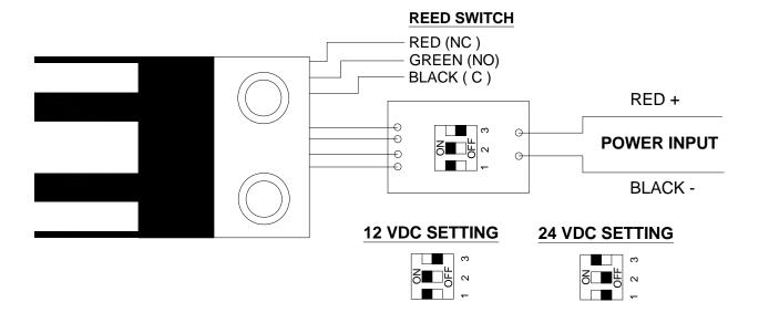
**WARNING:** The PCB Dip switch pin position must be set correctly before applying power to the lock, wrong pin setting will cause the PCB to fail. This will not be covered under warranty.
